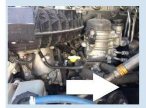
Gear Driven Power Steering Pump-
